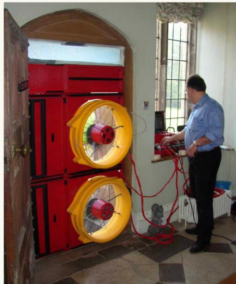
Blower door air permeability/leakage test
